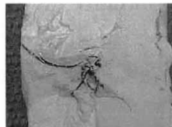
(c) Cement bentonite ( w/c=3 ) in OCR = 1 specimen
